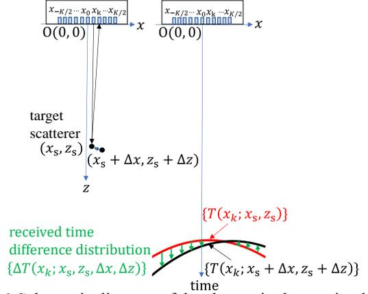
Fig. 1 Schematic diagram of the change in the received time distribution of scattered wave on elements caused by the 2-D displacement of the target.
