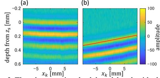
**Fig. 3** The element signals delayed by the ideal delay times  $T(x_k; x_s, z_s)$  and the received time difference  $\widehat{\Delta T}(x_k)$  (red line), (a) before and (b) after displacing the target.
