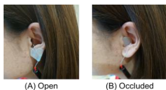
Fig. 2 Insertions of a probe microphone into the ear canal for the ECSP measurements.
