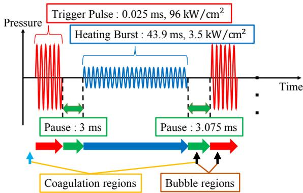
Fig. 3 HIFU irradiation sequence and timing of captured image used for image processing.
