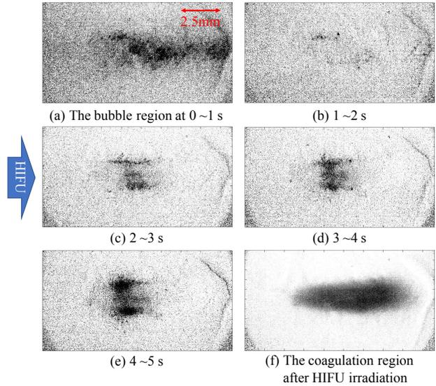
Fig. 5 Bubble and coagulation regions with the focal shift of 4 mm of the trigger pulse.
