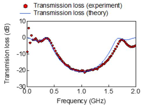
Fig. 4 Theoretical (blue line) and experimental (red plot) acoustic transmission loss of Bragg reflector.
