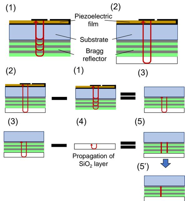
Fig. 1 The method to evaluate the sole mechanical properties of Bragg reflector
