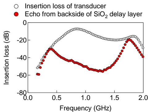
Fig. 3 Experimental insertion loss of transducer (white plot), and echo from back side of SiO<sub>2</sub> delay layer (red plot)
