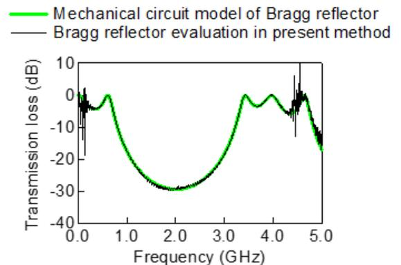
Fig. 2 Theoretical sole Bragg reflector property obtained by mechanical circuit (green line) and by the procedure of present method (black line).
