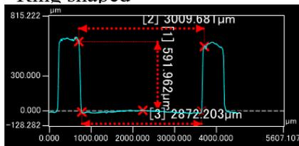
Fig.2 Photographs and profiling of 3D shapes  $\text{KNbO}_3$  piezoelectric films
