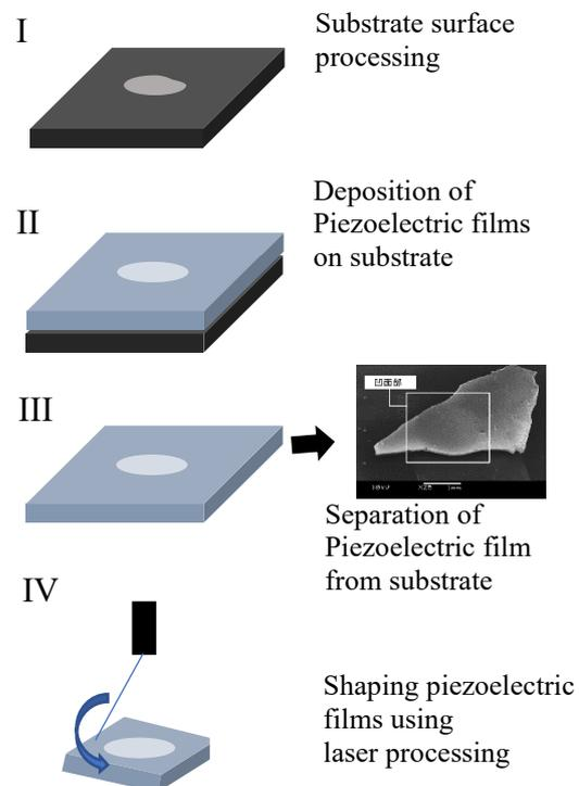
Fig.1 Schematic of concave piezoelectric film formation
