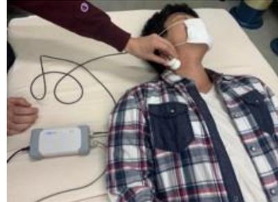
Fig. 1 Pulse wave measurement using a piezoelectric sensor.
