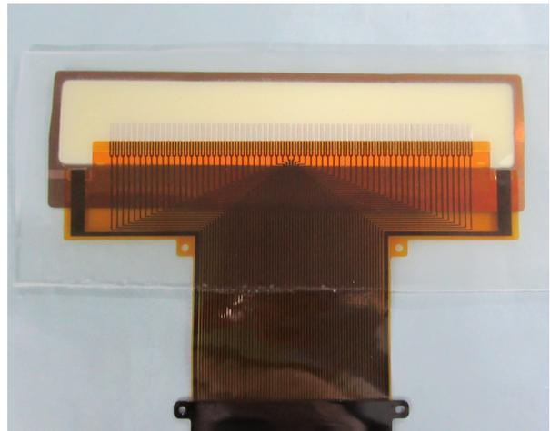
Fig. 1. Prototype of flexible ultrasonic array sensor.
