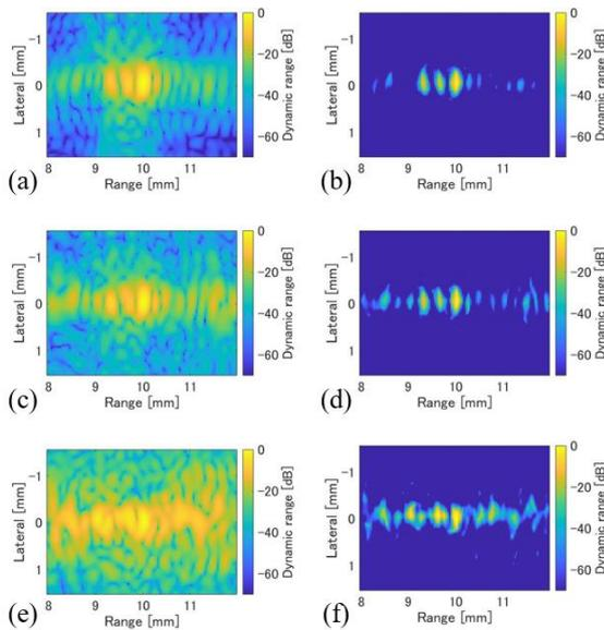
Fig 2. B-mode images. (a) and (b) are FM chirp, (c) and (d) are Method A, and (e) and (f) are Method B. The left column is DAS and the right column is weighted DAS.
