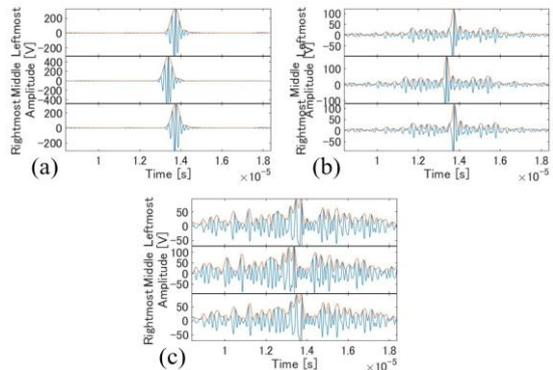
Fig 4. Compressed signals of (a) FM Chirp, (b) phased modulated signal separately, and (c) phase modulated signal simultaneously for 0 degree.
