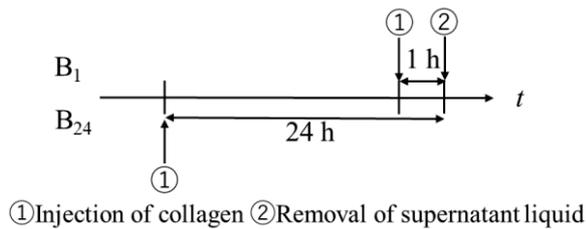
Fig.2 Time chart to prepare two basement membranes in flow channel.
