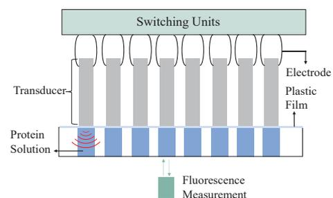
Fig. 1 Schematic illustration of the sonoreactor for amyloid fibril assay.
