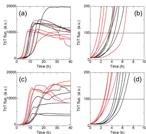
Fig. 2 Time-course curves of ThT fluorescence with SOS concentrations of (a) 0 mM and (b) is its enlarged view, (c) 4 mM and (d) is its enlarged view, respectively. Black and red lines show ThT curves with and without seeds, respectively.
