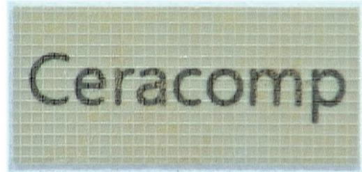
Fig. 6. Transparent 1-3 Single Crystal-Polymer Composite
