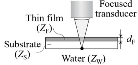
Fig. 1 Ultrasonic transmission system for recording the echo reflected on the back of the Si wafer through the photoresist film.
