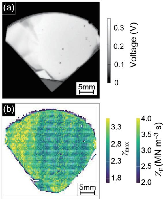
Fig. 2 (a) The acoustic image depicts the echo that is reflected from the backside of the wafer, certainly the area where the film was positioned on the top side. (b) The  $\gamma_{\max}$  image of the photoresist film constructed through signal processing (a), along with the scale bar of  $Z_F$ .
