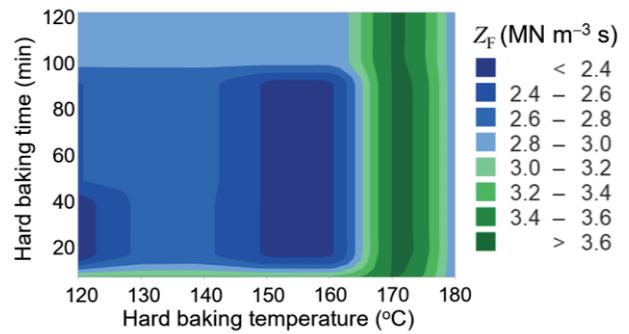
Fig. 3 The contour image of predicted  $Z_F$  by plotted on the hard baking temperature-time plane.
