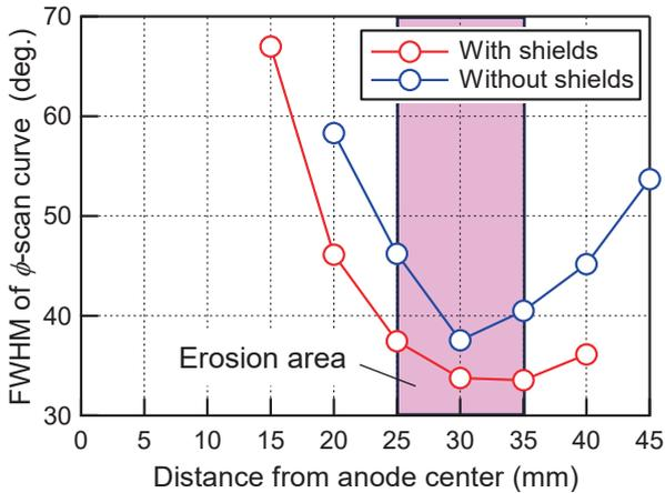
Fig. 2 FWHM of  $\phi$ -scan curve in ZnO films fabricated on Au electrode / SOI substrates as a function of distance from anode center.
