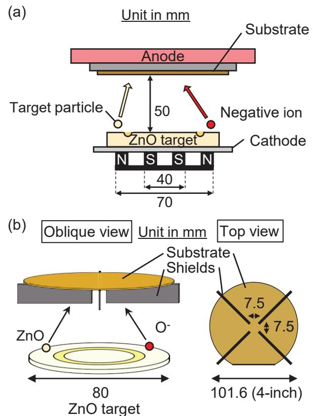
Fig. 1(a) RF magnetron sputtering apparatus and (b) schematic image of shields installation.
