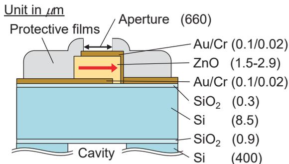
Fig. 3 Schematic image of shear-mode resonator.
