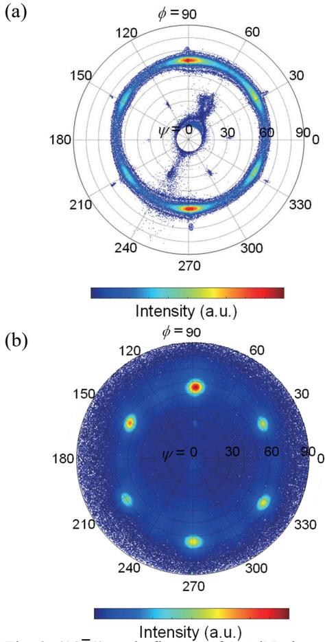
Fig. 2  $(10\bar{1}1)$  pole figures of ScAlN piezoelectric layer
