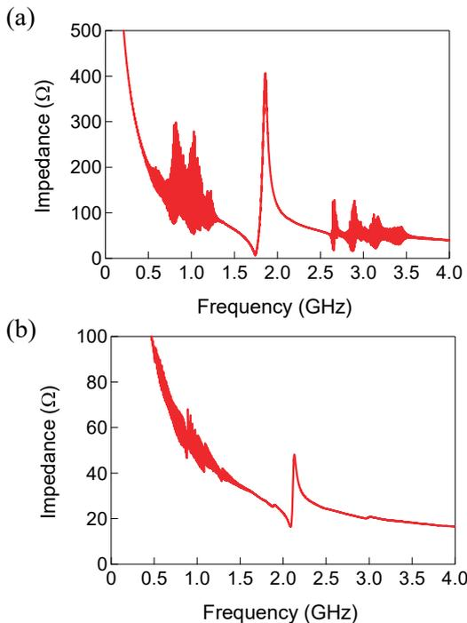
Fig. 3 Impedance characteristic of full-epitaxial SMR
