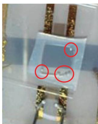
Fig. 6 After SAW excitation. Bubbles are observed.
