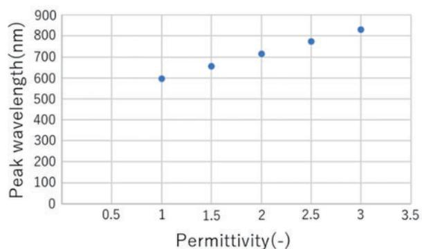
Fig. 4 LSPR peak wavelength as a function of permittivity (particle diameter: 15 nm, number of particles: 2, distance of particles: 1 nm)
