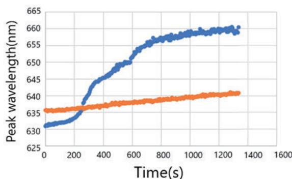
Fig. 2 LSPR peak wavelength of distilled water during SAW generation.
