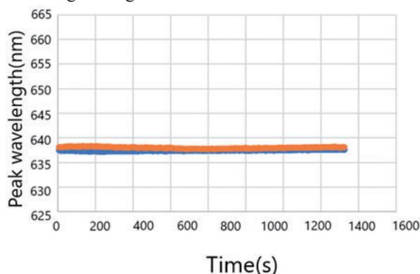
Fig. 3 LSPR peak wavelength of ultrapure water during SAW generation.
