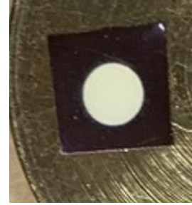
Fig.3 The sample fabricated on SUS foil and 47 \text{ }\mu\text{m} of film thickness for scanning SEM
