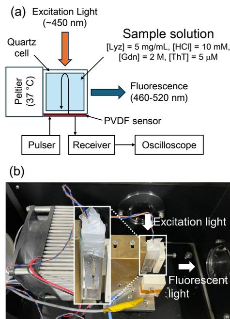
Fig. 1 (a) Schematic illustration and (b) picture of the experimental setup for simultaneous measurement of ultrasonic and fluorescence spectra.
