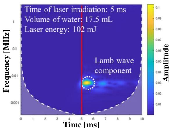
Fig. 2 A scalogram of time waveform measured by the sensor with piezoelectric film/silicon rubber structure.
