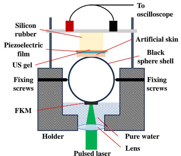
Fig. 1 Cross-sectional view of spherical shell fixing holder with condenser lens.
