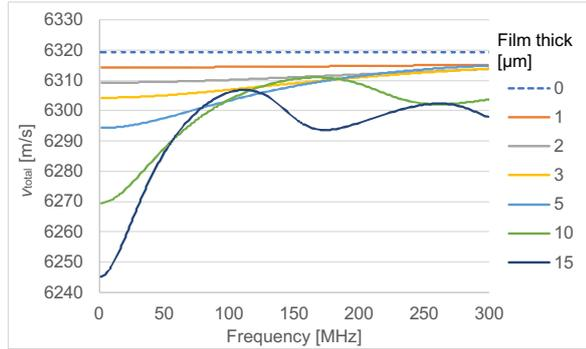
Fig. 3 Calculation results of  $v_{total}$  for Ta<sub>2</sub>O<sub>5</sub> film on Z-cut quartz substrate with 2 mm thick.
