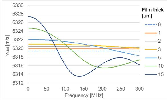
Fig. 2 Calculation results of  $v_{total}$  for SiO<sub>2</sub> glass film on Z-cut quartz substrate with 2 mm thick.
