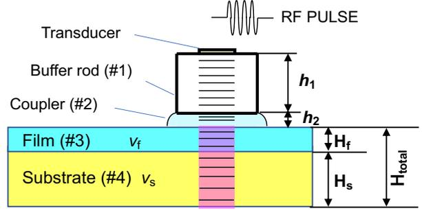
Fig. 1 Configuration of bulk wave velocity measurement for a thin film on a substrate using the PW-UMC system.
