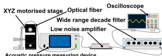
Fig. 2 Acoustic pressure measurement system.
