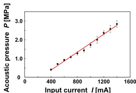
Fig. 3 Acoustic pressure against input current. (n = 10, mean  $\pm$  S.D.).
