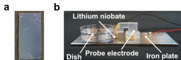
Fig. 1 Ultrasound irradiation device. (a) Lithium niobate. (b) Irradiation device.
