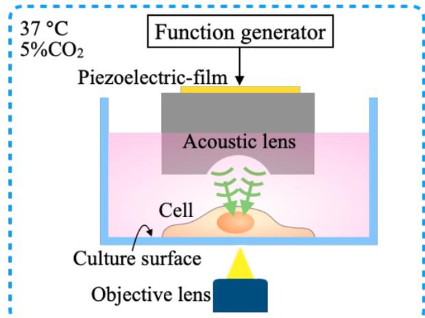
Fig. 1 The developed ultrasound system for the nucleus stimulation in culture environment.
