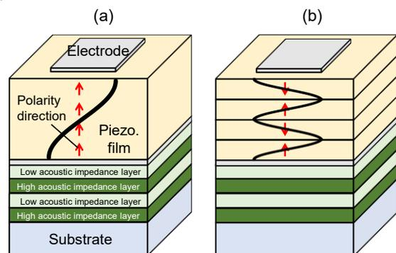
Fig. 1 (a) single-layer film and (b) polarization inverted film BAW resonators (SMR structure)
