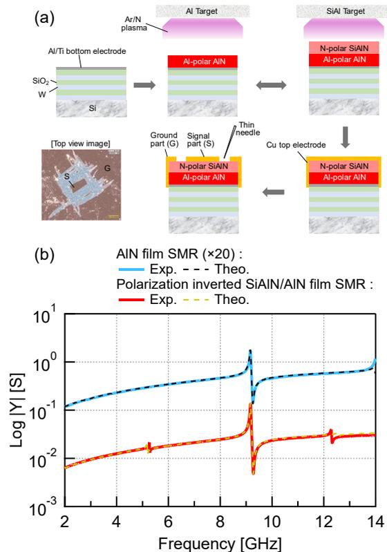
Fig. 3 (a) Fabrication process and (b) admittance frequency characteristics for the single layer AlN film and two-layer polarization-inverted SiAlN/AlN film SMRs.
