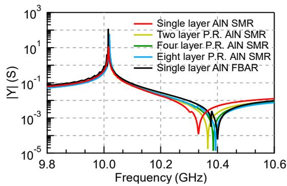
Fig. 2 Admittance frequency characteristics of polarization inverted AlN film SMRs analyzed by FEM.
