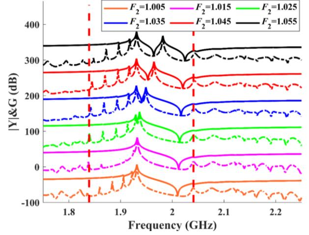
Fig. 5 Variation of  $|Y|$  and  $G$  with  $F_2$  when  $N_{IDT2}=5$  and  $F_r=0.975$ . Red broken lines: reflector stopband edges.
