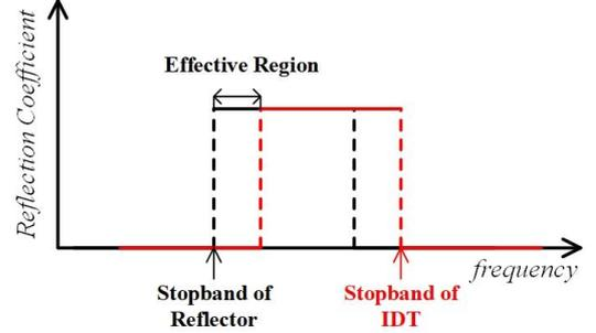
Fig. 2 Stopband of reflector and IDT
