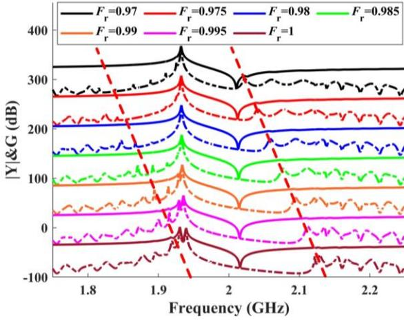
Fig. 3 Variation of  $|Y|$  and  $G$  with  $F_r$  when  $F_2=1.01$  and  $N_{IDT2}=7$ . Red broken lines: reflector stopband edges.
