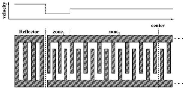
Fig. 1 ‘Piston-like’ design and SAW velocity profile
