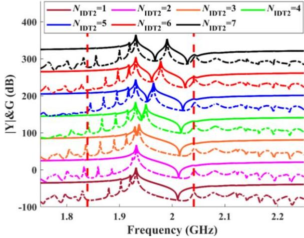
Fig. 4 Variation of  $|Y|$  and  $G$  with  $N_{IDT2}$  when  $F_2=1.025$  and  $F_r=0.975$ . Red broken lines: reflector stopband edges.
