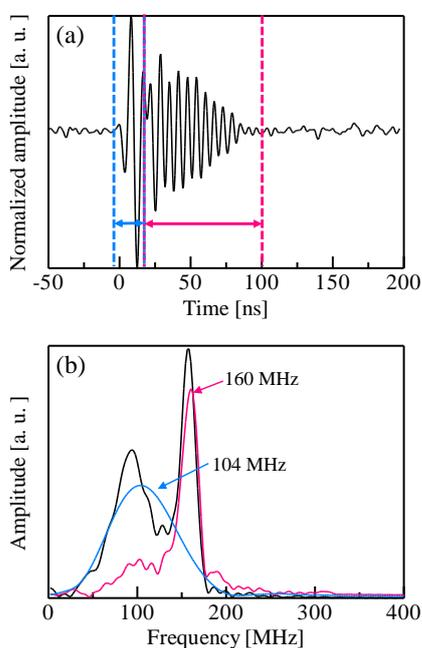
Fig. 2 (a) The representative waveform of reflected wave from the culture surface detected by the self-made acoustic probe, and (b) the corresponding FFT spectra. The blue and magenta spectra are obtained by performing FFT analysis on the waveform in the ranges indicated by the arrows of the same colors as the spectra. The frequency value is the frequency peak on each spectrum.
