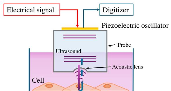
Fig. 1 Experimental setup for obtaining spectroscopic acoustic images of live cells.
