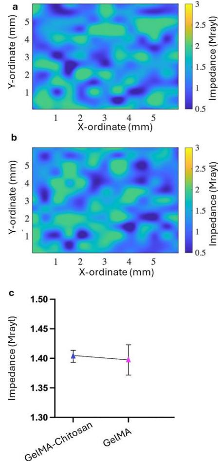
Fig. 2 Acoustic Impedance of- a) GelMA-chitosan, b) GelMA, and c) their comparison.
