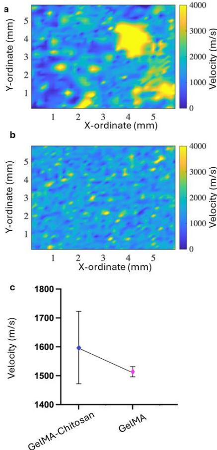
Fig. 3 Longitudinal velocity of - a) GelMA-chitosan, b) GelMA, and c) their comparison.
