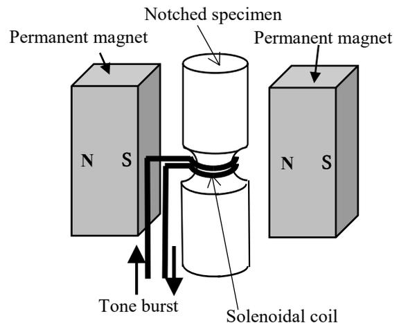
Fig.2 The Lorentz-force mechanism causes an axial-shear-wave EMAT
