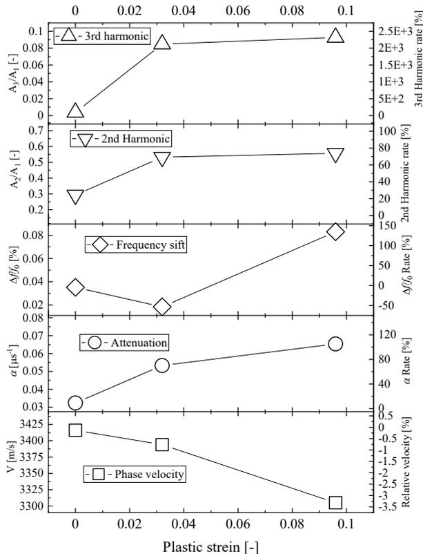
Fig.2 The relationship with plastic strain and ultrasonic characterizations in U- notch specimen.
