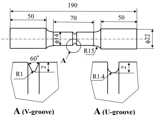
Fig.1 Shape of 2 types of notched samples
