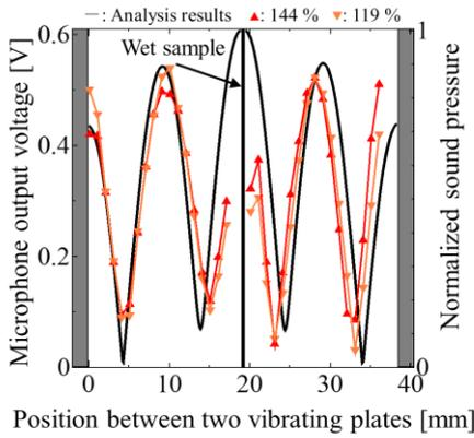
(a) Placed at sound pressure anti-node position.
