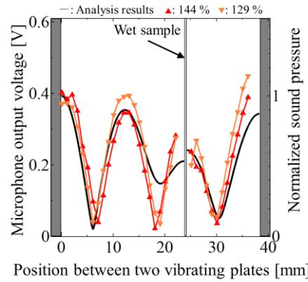
(b) Placed at sound pressure node position.
