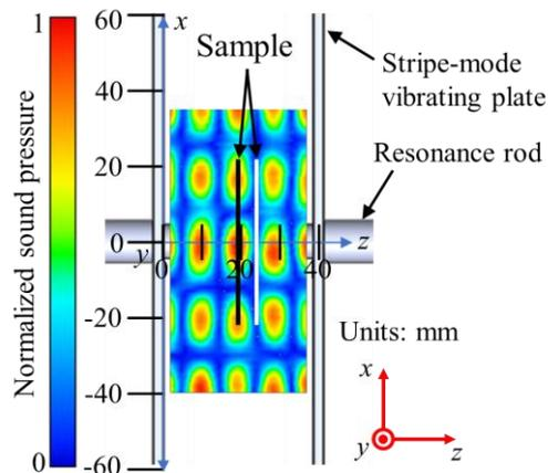
Fig. 3 Measured sound pressure distribution of standing wave sound field with no sample plate.
