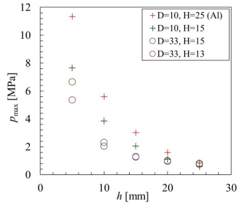
Fig. 4 Maximum sound pressure in the cavity  $p_{\max}$  (acrylic cylinder) vs. gap  $h$ .
