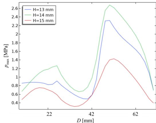
Fig. 5 Maximum sound pressure in the cavity  $p_{\max}$  vs. Diameter of the acrylic cylinder  $D$  ( $h=25$  mm).
