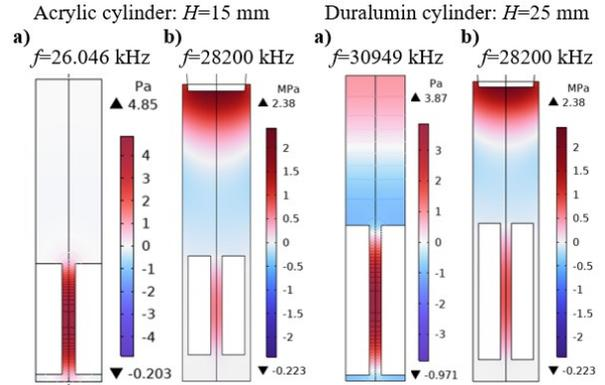
Fig. 3 Sound pressure distributions obtained by a) eigenfrequency analysis and b) frequency domain analysis for  $D=10$  mm,  $d=2$  mm,  $h=25$  mm, and  $A=20$   $\mu$ m.
