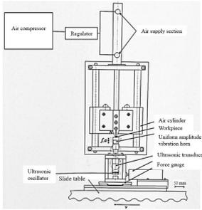
Fig. 2 Ultrasonic vibration friction experimental equipment.
