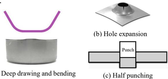
Fig. 4 Examination of application method to sheet metal forming.
