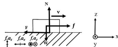
Fig. 1 Ultrasonic vibration direction.
