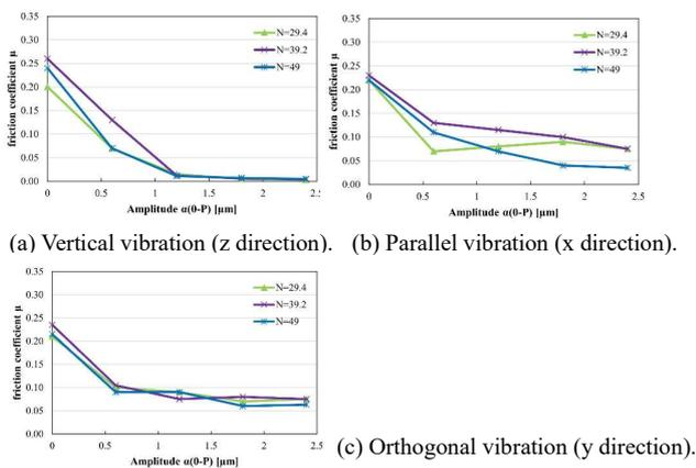
Fig. 3 Relationship between ultrasonic vibration amplitude and friction coefficient
