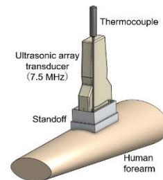
Fig. 1 Experimental setup for UVC imaging of the human forearm.
