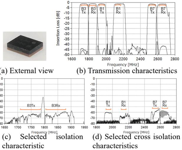
Fig. 4 External view and measured characteristics of fabricated hexaplexer.
