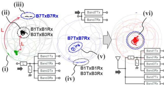
Fig. 3 Antenna matching circuit for hexaplexer.
