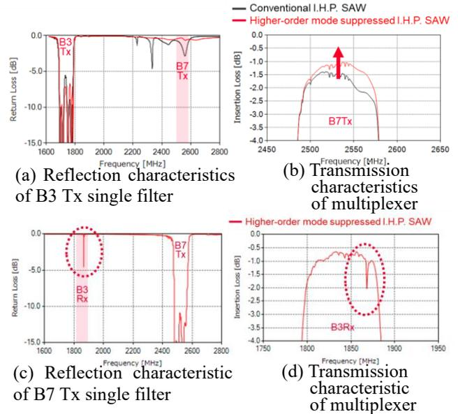
Fig. 1 Simulated characteristics of single filter state and multiplexer State.
