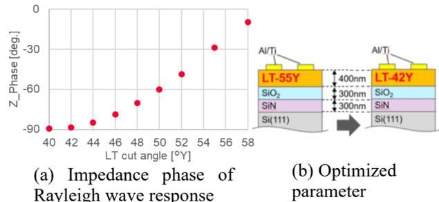
Fig. 2 Variation of intensity of Rayleigh wave response on LT cut angle and the optimized parameter.
