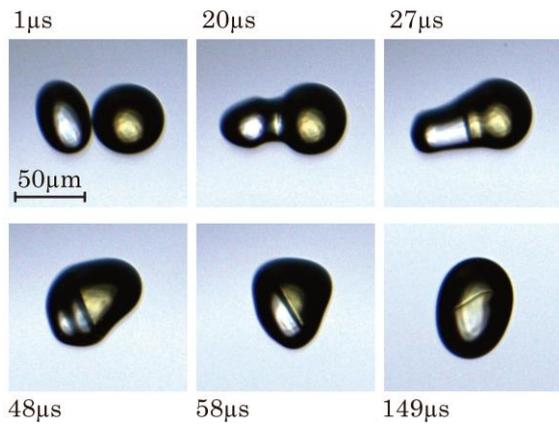
Fig. 3 Collision of a distilled water droplet from the left and a soy sauce droplet from the right. Each droplet is ejected from a nozzle with the diameter of 50  $\mu\text{m}$ .
