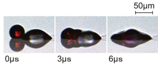
Fig. 1 Dye-doped ethanol droplet on the left colliding on a glass plate with distilled water droplet on the right. In this figure, we can see the mirror images of actual droplets reflected on the glass surface on the lower side of each photo.
