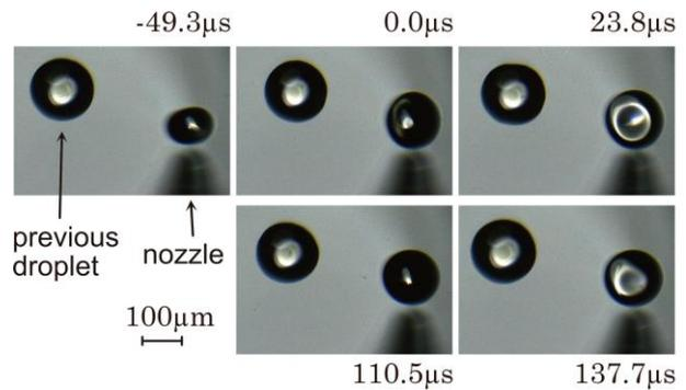
Fig. 5 Photographs of a droplet of distilled water landing on a glass substrate, taken from the back side of the substrate. The nozzle diameter is 50  $\mu\text{m}$ . The time when the drop landed on was set as 0  $\mu\text{s}$ .
