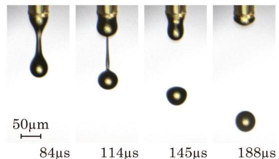
Fig. 2 Photos of generating a droplet of Yamami Brewery's Tamari Soy Sauce. The nozzle is  $\phi 50 \mu\text{m}$ .
