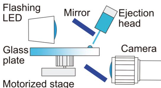
Fig. 4 Schematic view of our droplet observation system in this study using microscopic strobe technology.
