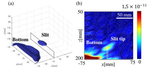
Fig. 4 3D imaging result of the slit obtained by low-frequency PLUS. (a) 3D view (b) B-scan ( $xz$ -plane at  $y = 0$  mm) image extracted from (a).
