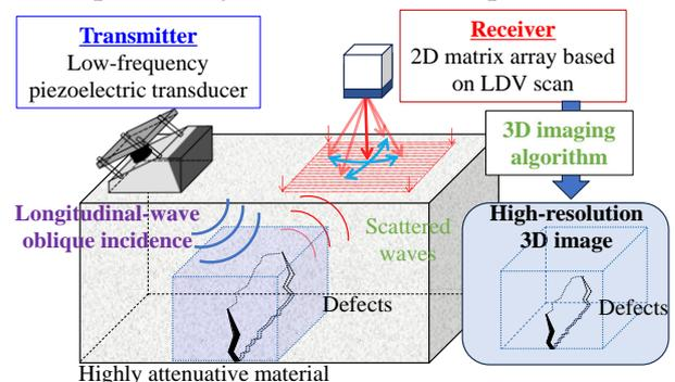
Fig. 1 Schematics of low-frequency PLUS.
