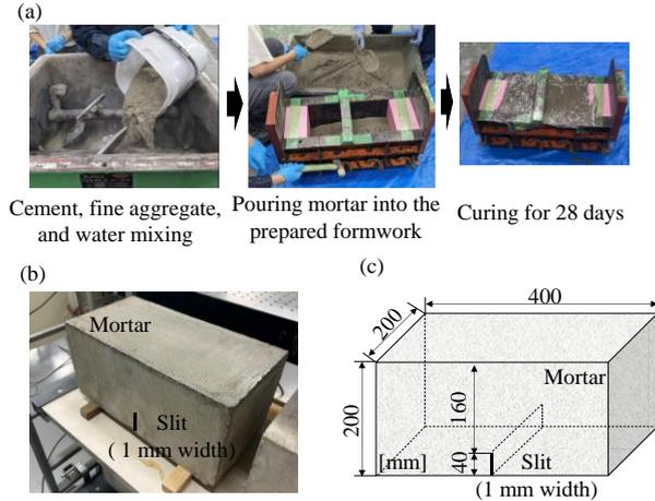
Fig. 2 Mortar sample with a slit (a) Preparation flow, (b) photo, and (c) design.
