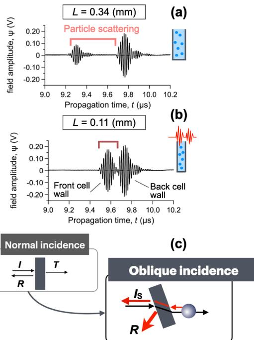
Fig. 1 Examples of reflected echoes from (a) a thick cell ( $L=0.34$  mm) and (b) a thin cell ( $L=0.11$  mm). (c) schematic figure of the oblique incidence setup employed in this study.
