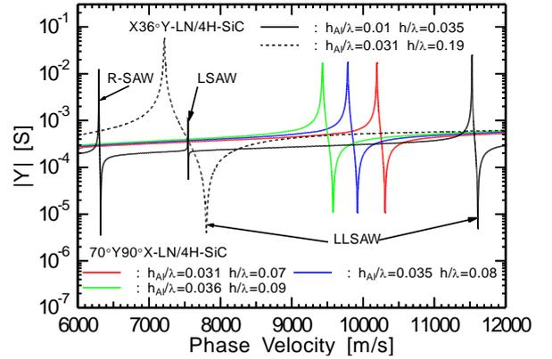
Fig. 4 Simulated resonance properties on  $70^\circ\text{Y}90^\circ\text{X-LN}/4\text{H-SiC}$ .
