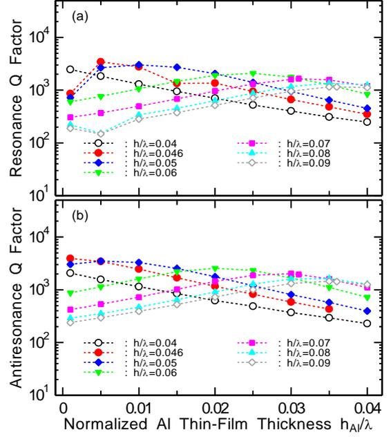
Fig. 3 Al thin film thickness dependences of (a) resonance and (b) antiresonance  $Q$  factors of LLSAW.
