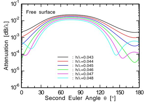
Fig. 1 Calculated attenuation of LLSAW on Rot.Y90°X-LN /4H-SiC.
