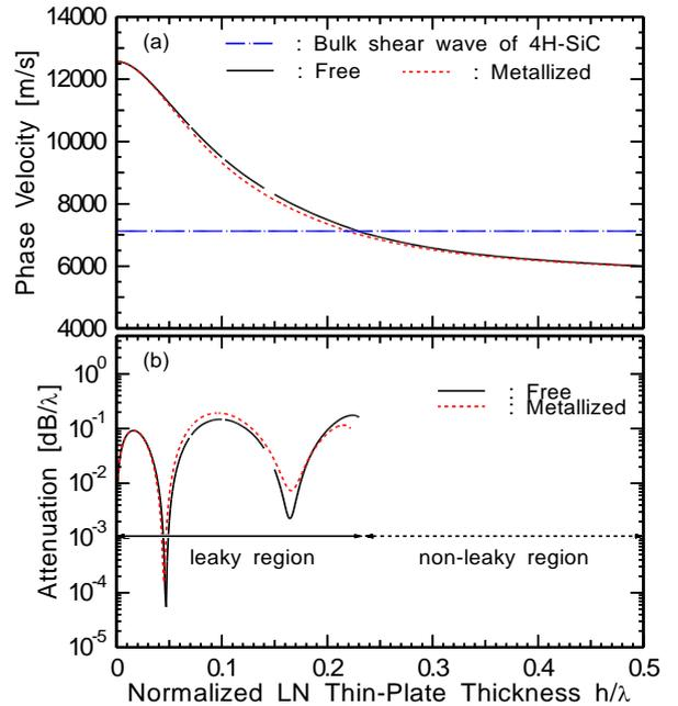
Fig. 2 Calculated propagation properties for (a) phase velocity and (b) attenuation of LLSAW on 70°Y90°X-LN /4H-SiC.
