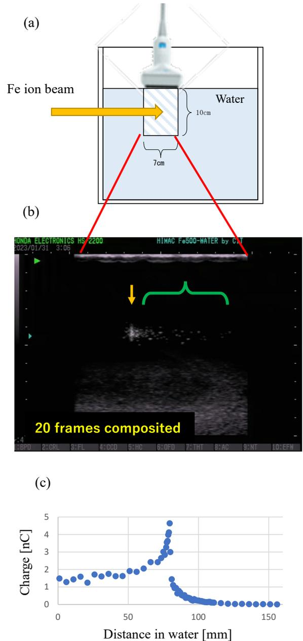
Fig. 1: Illustration showing an overview of the experimental setup (a), a frame composite of the ultrasound echo animation of the Fe beam irradiation (b), and the results of the dose measurements taken with the Marcus ionization chamber against the beam (c).
