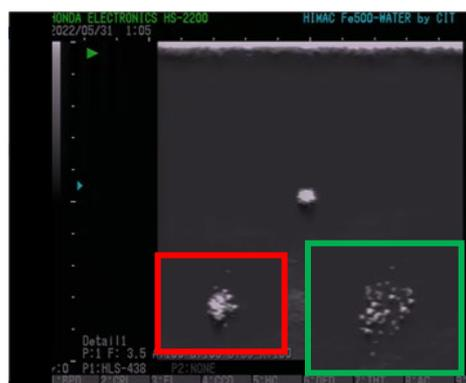
Fig. 2: An image of one frame of the ultrasound echo image when the beam intensity was fixed at  $1.0 \times 10^8$  ppp and the spot size of  $\phi 5$  mm and cropped images of the spot size of  $\phi 10$  mm (red frame) and  $\phi 20$  mm (green frame) are superimposed for comparison.
