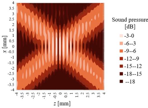
Fig.2 Distribution of sound pressure in the interference field with the angles of  $\theta = 40$  deg and  $\varphi = 0$  deg.
