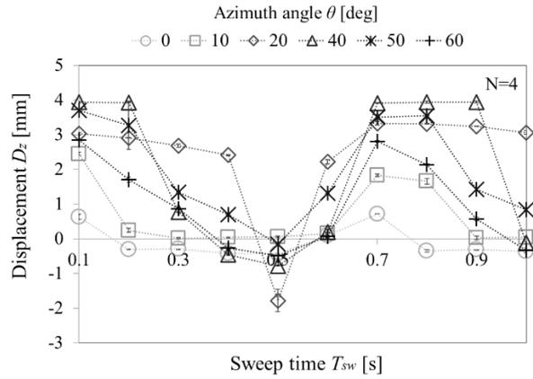
Fig.4 Relationship between the sweep time and the catheter displacement using phase sweeping.
