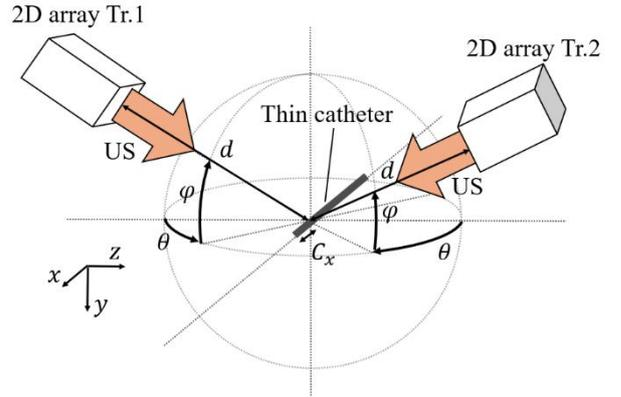
Fig.1 Experimental setup to bend thin catheter with two 2D array transducers.
