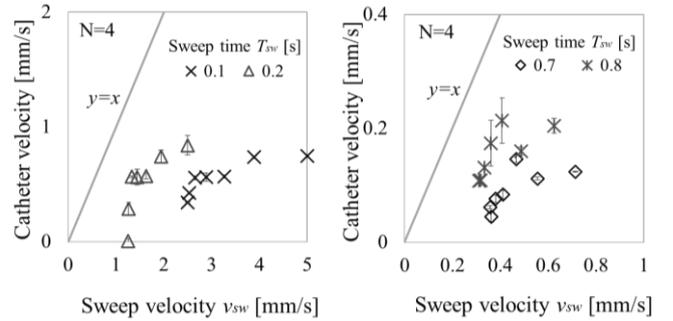
Fig.5 Relationships between the sweep velocity and the catheter velocity when the sweep time was  $T_{sw} = 0.1, 0.2$  s (left) and  $T_{sw} = 0.7, 0.8$  s (right).
