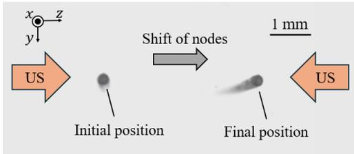
Fig.3 Observation of the tip of the catheter before and after the ultrasound irradiation.
